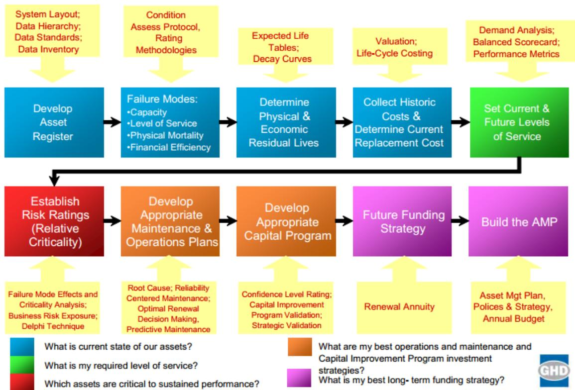
Figure 3: 10 Steps process to reach stormwater asset management program (City of San Diego, 2013)
